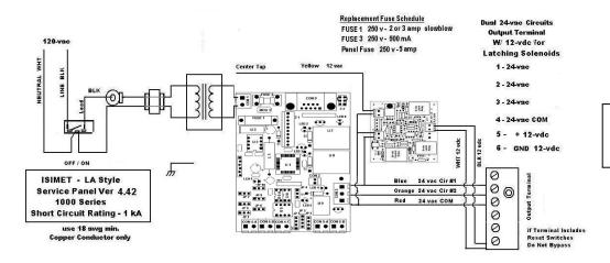
W/ 24-vac Output and W/ 12-vdc Output
